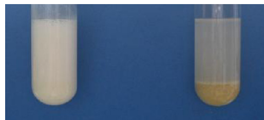
Fig. 2. Photographs of 3 (GFQAS) catalyzed reaction in water. The emulsion of catalyst and reagents formed at the beginning of reaction (I) and the product precipitated after the reaction finished (II). Upper layer: the catalytic mother solution; lower layer: the crude product.
